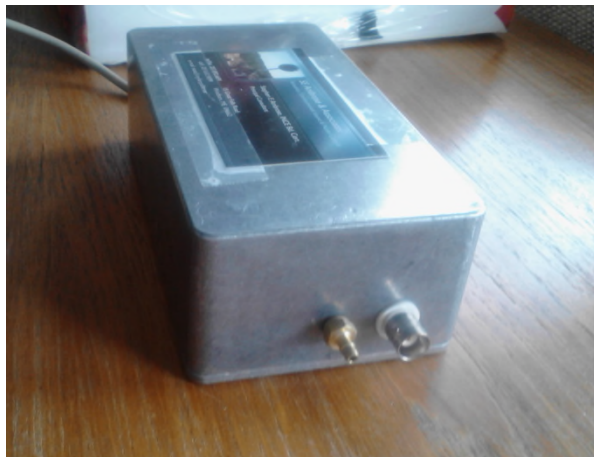
Figure 7-Infiltec-20 micro barometer. Resolution: 0.001 Pascals from 0.1 to 20 Hz. Data sampled 50 times a second in signed 16bit integers. Range: \pm 25 Pascals.
